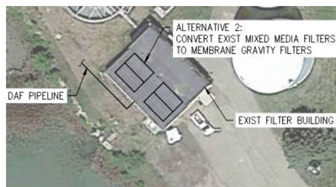
Figure 2: Alt #2 – Convert Existing Filters to MGFs
