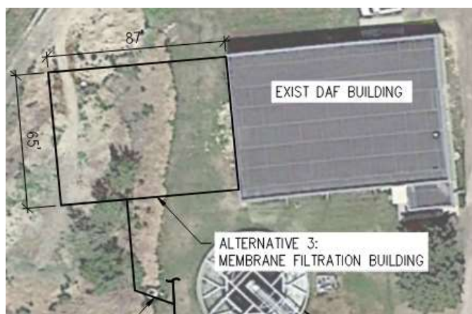
Figure 3: Alt #3 - Construct New Membrane Filtration System
