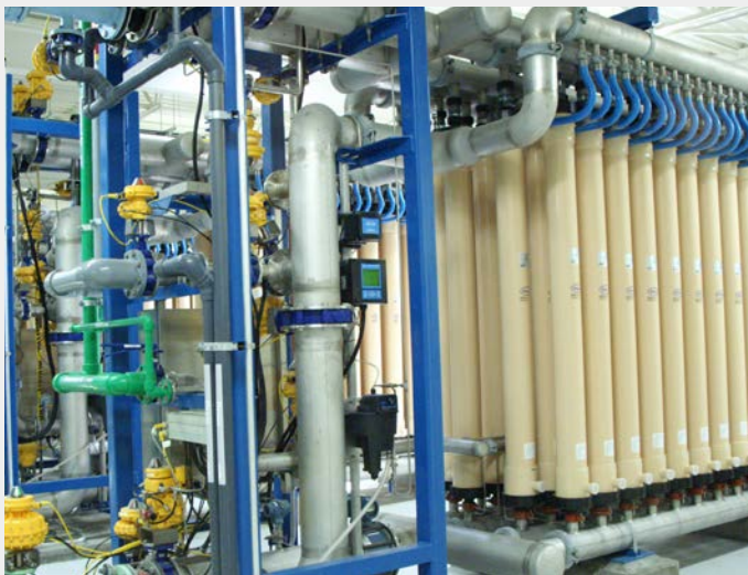
Typical membrane racks can provide significant treatment capacity in a compact footprint but will require significant valves, instruments, and ancillary equipment.
