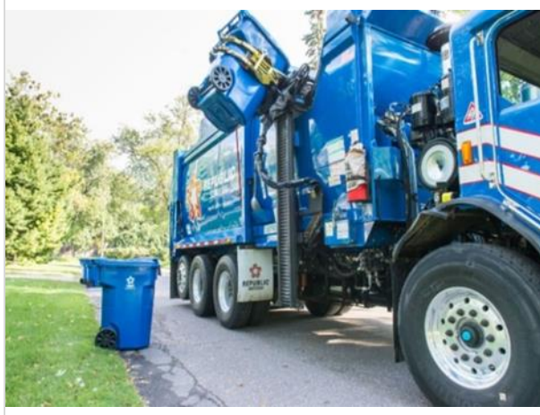
Figure 12. Automated Side Load Collection. Provides a cleaner, safer, more efficient residential collection.
